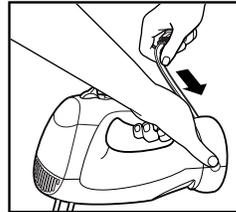
**NOTE:** If the cord jams during storage, unwind slightly and then press cord release button and guide the cord into place.
