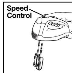
set at **0** (OFF) push straight down on the speed control.
