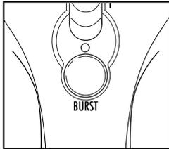
**NOTE:** Do not use Power Burst for more than two minutes at a time or motor may overheat.
