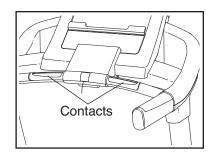
To measure your heart rate, stand on the foot rails and hold the contacts—avoid moving your hands. When your pulse is detected, several dashes will appear and then your heart rate will be shown. For the most accurate heart rate reading, continue to hold the contacts for about 15 seconds.
