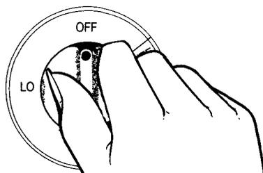
To turn a burner off, turn the knob clockwise, as far as it will go, to the OFF position.
