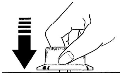
Push the control knob in and turn it counterclockwise to LITE.
