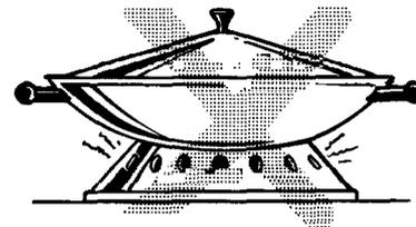
over the burner grate may cause the burner to work improperly resulting in carbon monoxide levels above allowable current standards. This could be dangerous to your health. Do not try to use such woks without the ring. You could be seriously injured if the wok tipped over.
