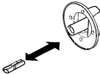
To replace knob, match the "D" shaft on the knob to the "D" shaft on the stem. Do not force the knob.
