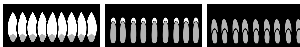
A–Yellow flames Call for service B–Yellow tips on outer cones Normal for LP gas C–Soft blue flames Normal for natural gas
