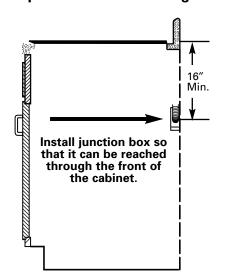
**AIMPORTANT:** The junction box must be located where it will allow considerable slack in the conduit for serviceability.
