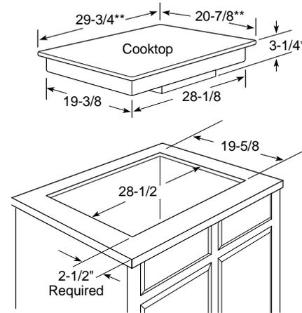
\*Depth of unit at conduit location (rear) is 6-1/4"
