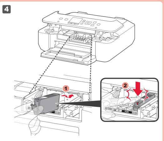
Insert and push down the ink tank firmly until it snaps into place.
