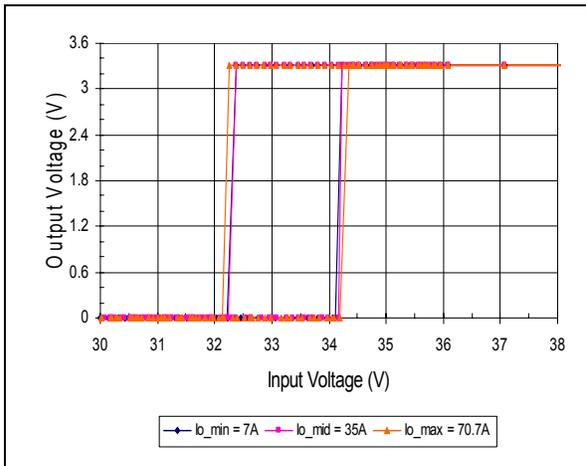
Typical Output Voltage vs. Input Turn-on and Turn-off Voltage at Ta=25C
