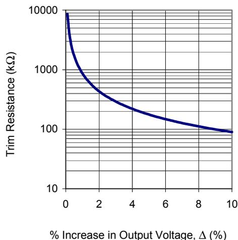
The value of  $V_{ref}$  can be found in the Electrical Data section of this data sheet. The maximum power available from the power module is fixed. As the output voltage is trimmed up, the maximum output current must be decreased to maintain the maximum rated power of the module. It is also desirable to slightly increase the input voltage while trimming up the output with heavy load current.
