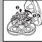
**3** Turn the black 3-pronged locking bracket counterclockwise (1) and remove the retaining frame (2).
