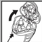
**2** Press the razor head release button to open the Razor Head Assembly.
