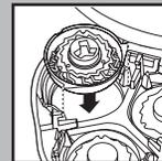
**6** Replace the set back into the Razor Head Assembly so that the “wings” on the comb fit within the brackets located towards the center of the Assembly.
