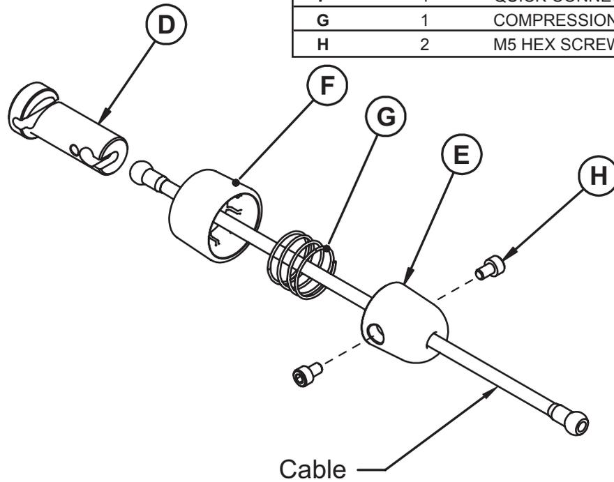
Slide Mechanism to insert or Exchange Handles
