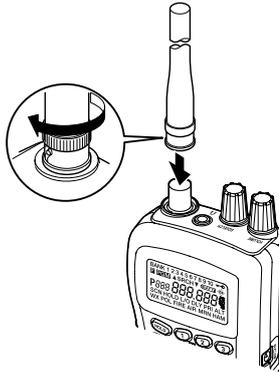
To attach the supplied flexible antenna to the connector on the top of your scanner, align the slots around the antenna's connector with the tabs on the scanner's BNC connector. Then slide the antenna's
