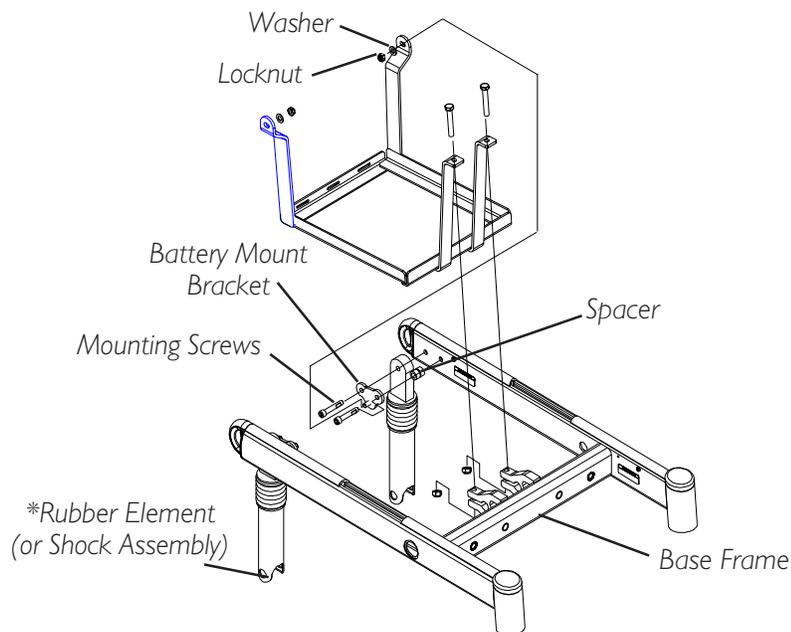
*\*NOTE: Illustration depicts rubber element. Battery Mount Brackets remove in the same manner for the shock assembly.*
