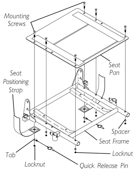
*NOTE: Illustration shows standard frame only for clarity. The seat pan removes/installs onto the ASBA the way.*
