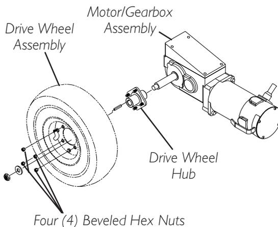
**WHEELCHAIRS BUILT BEFORE 1/26/04 ONLY**
