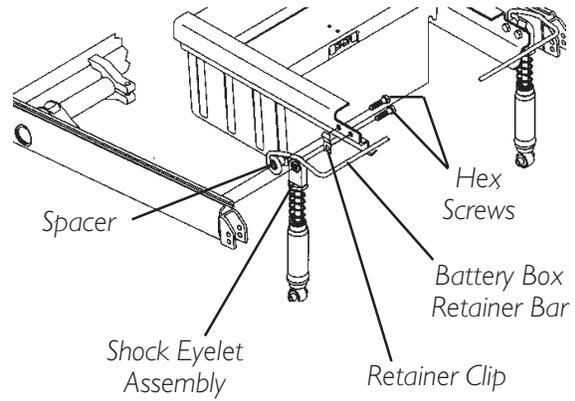
*NOTE: Shock exploded away for clarity. There is no need to remove shock from suspension arm.*
