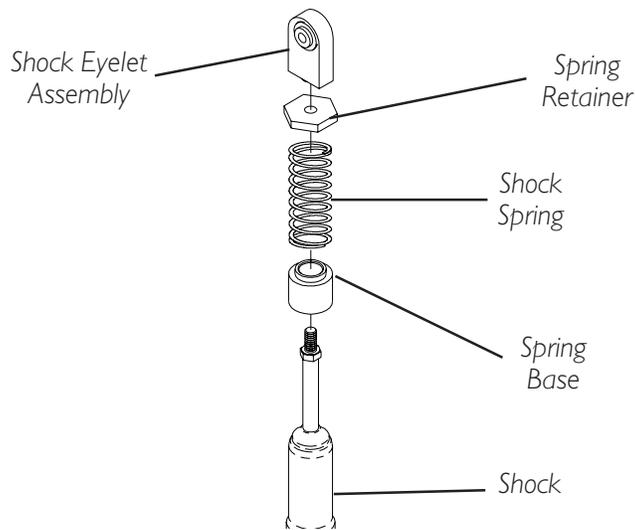
**FIGURE 8 - SHOCK SPRING REPLACEMENT**
