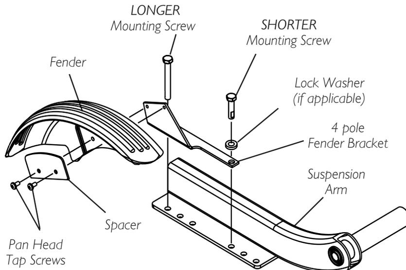
**FIGURE 12 - INSTALLING/REMOVING FENDERS - 4 POLE MOTORS**
