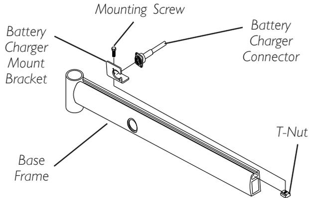
**FIGURE 4 - REPLACING BATTERY CHARGER BRACKET AND T-NUT**
