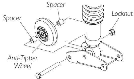
**FIGURE 17 - ANTI-TIPPER WHEEL REPLACEMENT****REMOVING/INSTALLING THE 3-INCH ANTI-TIP ASSEMBLY (FIGURE 18)**
