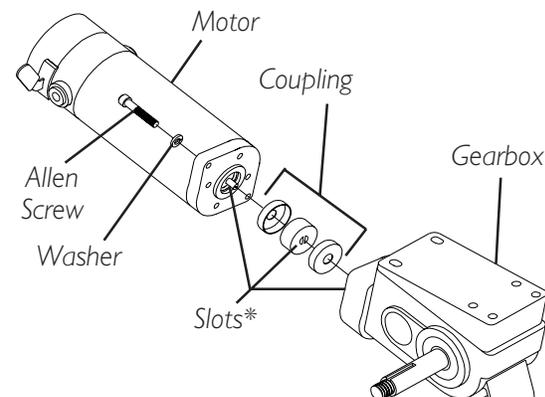
*\*NOTE: The slots on coupling of motor, the slots on the coupling and the slots on the gearbox must line up for proper installation*
