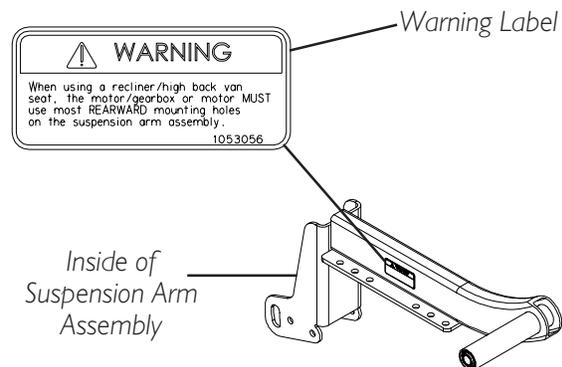
**FIGURE 7 - INSTALLING/
