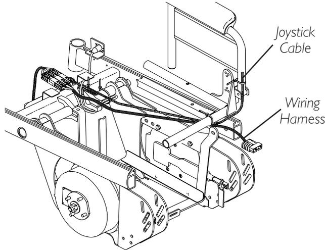
*NOTE: Illustration depicts gearless/brushless motor. Wiring harness is secured to the rear of the seat frame in the same manner for wheelchairs with conventional motor/gearbox assembly.*
