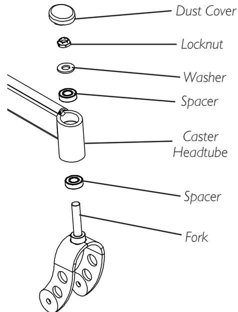
**FIGURE 8 - REPLACING FORKS**
