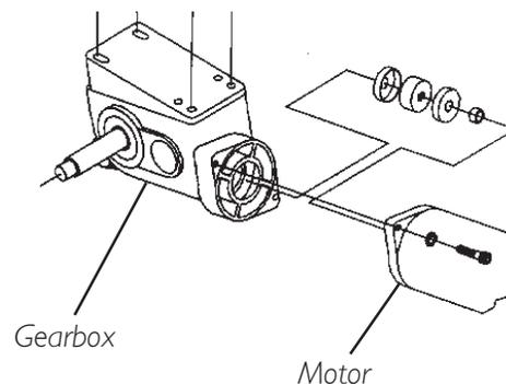
**FIGURE 9 - REMOVING/INSTALLING GEARBOX**
