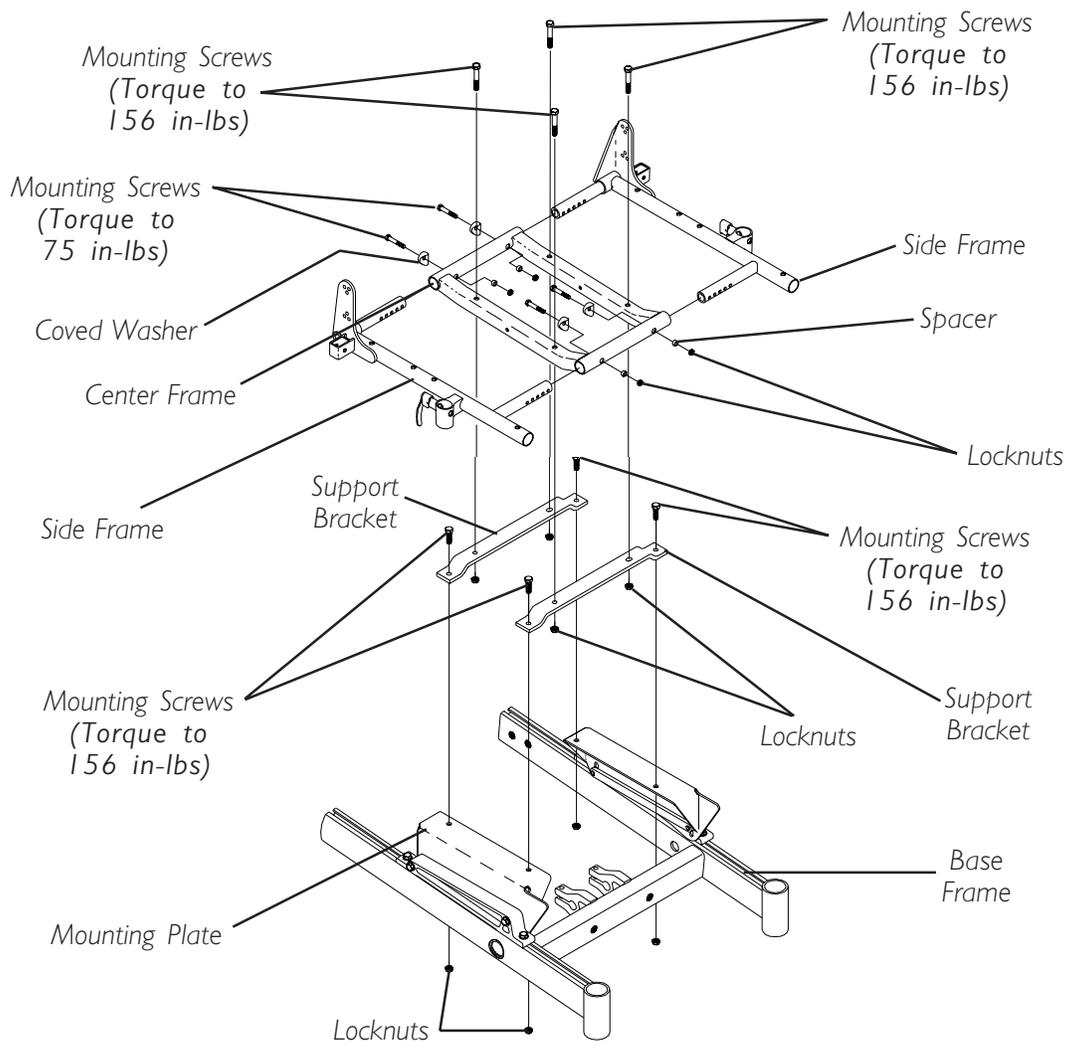
**FIGURE 6 - INSTALLING/REMOVING ASBA SUBASSEMBLY AND/OR COMPONENT REPLACEMENT**
