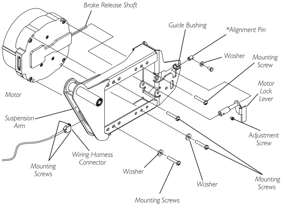
*\*NOTE: Alignment pin exploded away suspension arm for clarification purposes only.*
