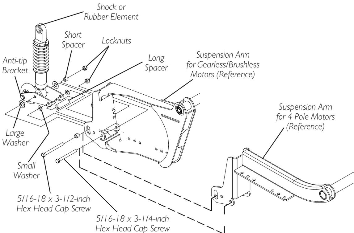
**FIGURE 18 - REMOVING/INSTALLING THE 3-INCH ANTI-TIP ASSEMBLY**
