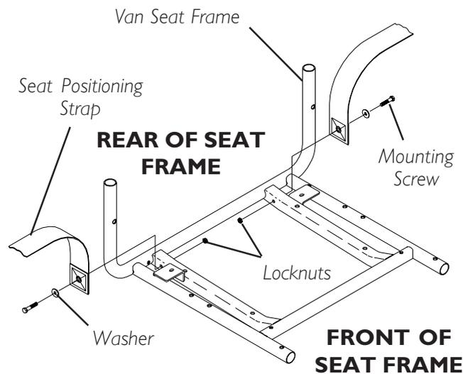
**FIGURE 1 - REPLACING VAN SEAT POSITIONING STRAP**
