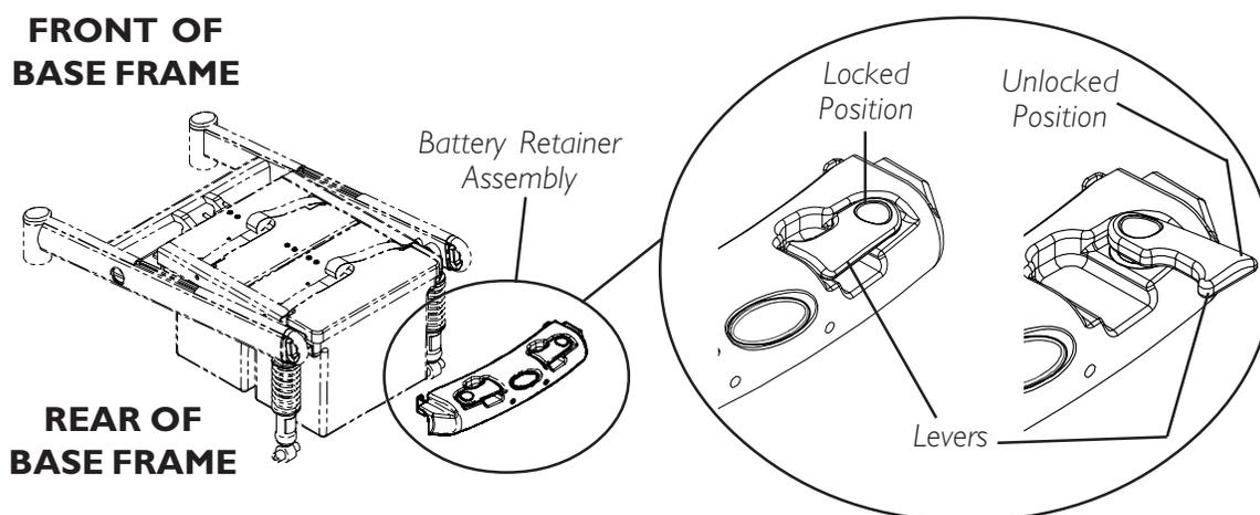
**FIGURE 8 - REMOVING/INSTALLING BATTERY BOXES - GROUP 24
