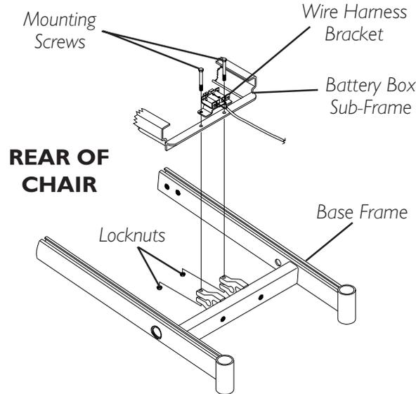
**DETAIL "B" - WHEELCHAIRS WITH MOTOR/GEARBOX ASSEMBLY**
