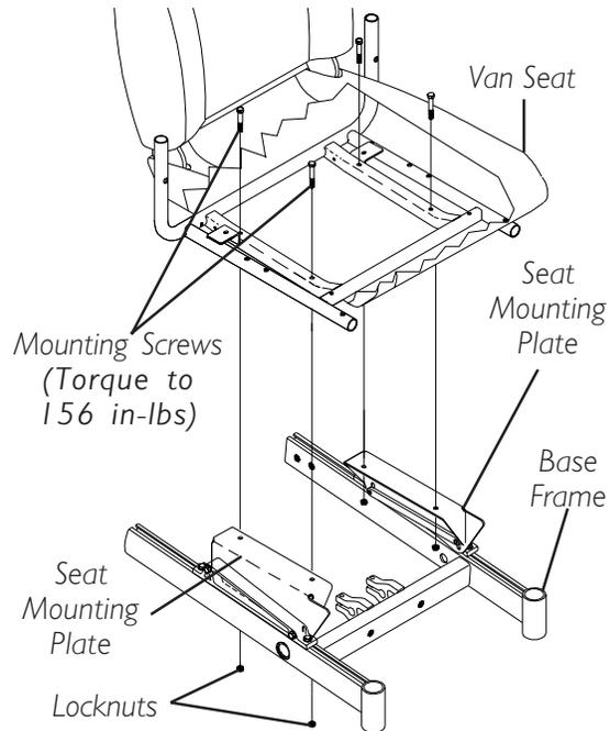
**FIGURE 7 - REMOVING/
