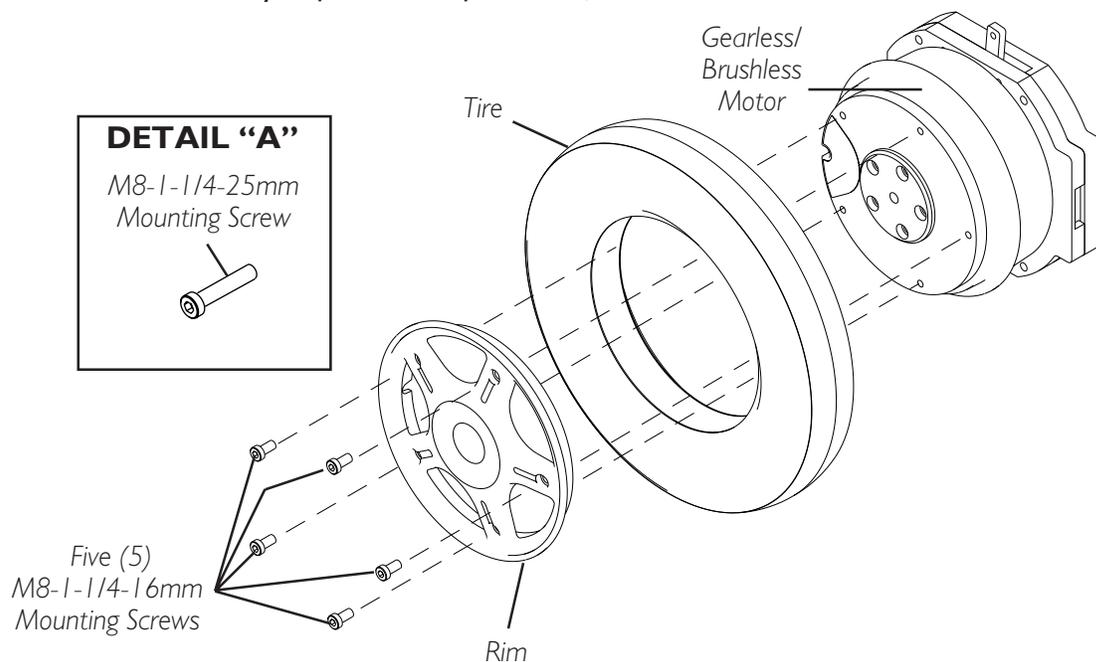
**FIGURE 6 - REMOVING/INSTALLING THE RIM AND/OR TIRE**
