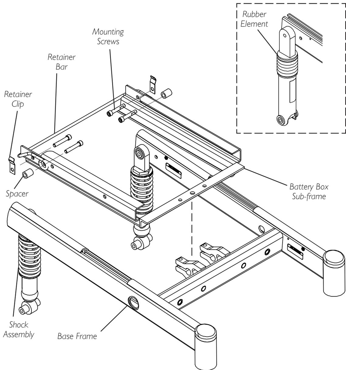
FIGURE I - REPLACING BATTERY BOX RETAINER BAR/RETAINER CLIP
