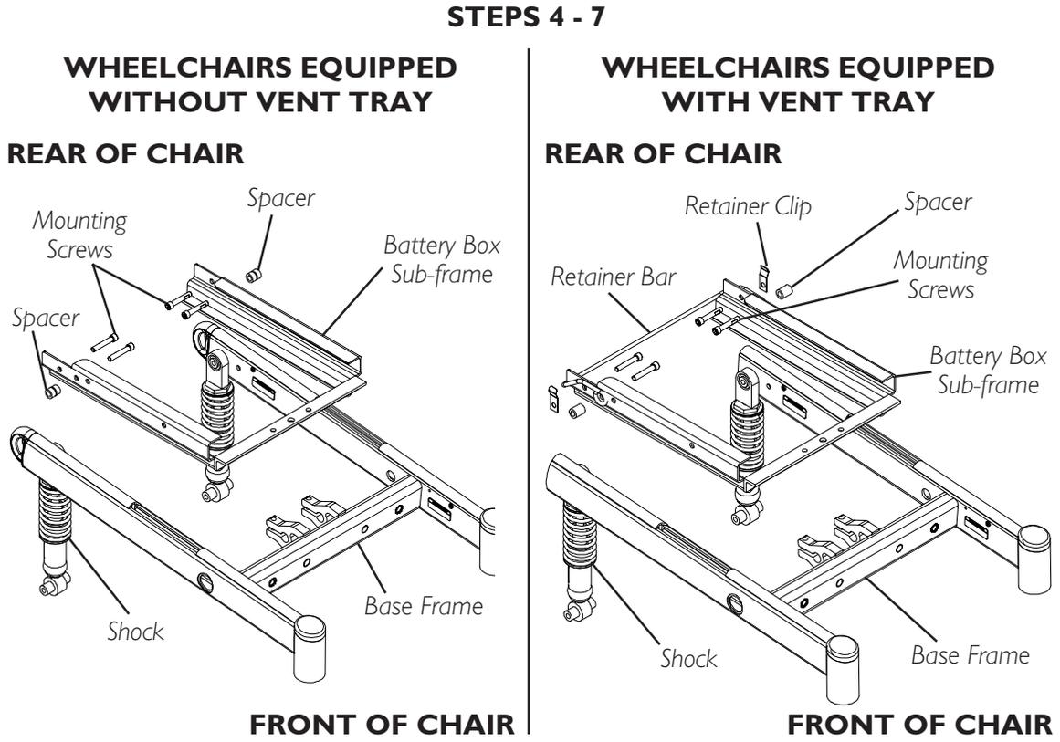
**FIGURE 4 - INSTALLING GROUP 24 COMPONENTS**
