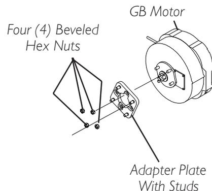
**FIGURE 4 - REMOVING/INSTALLING THE ADAPTER PLATE WITH STUDS**
