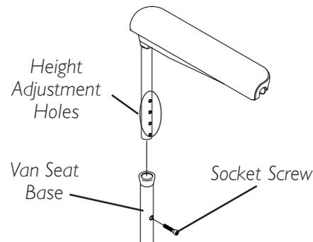
**FIGURE 1 - PREPARATION FOR REMOVING/INSTALLING SEAT FRAME (STANDARD FRAME, ADJUSTABLE FRAME, AND VAN SEAT)**
