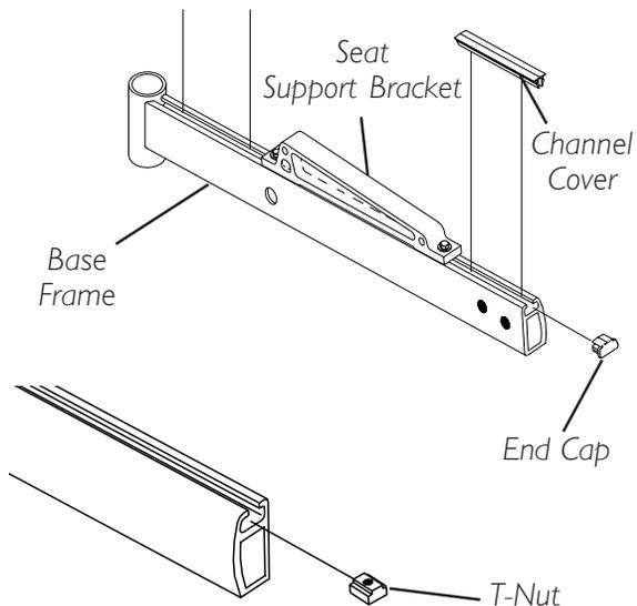
**FIGURE 3 - REPLACING SEAT SUPPORT BRACKET T-NUTS**
