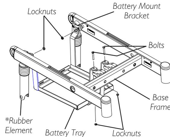
*\*NOTE: Illustration depicts the rubber element. Battery Box Tray removes in the same manner for shock assembly.*
