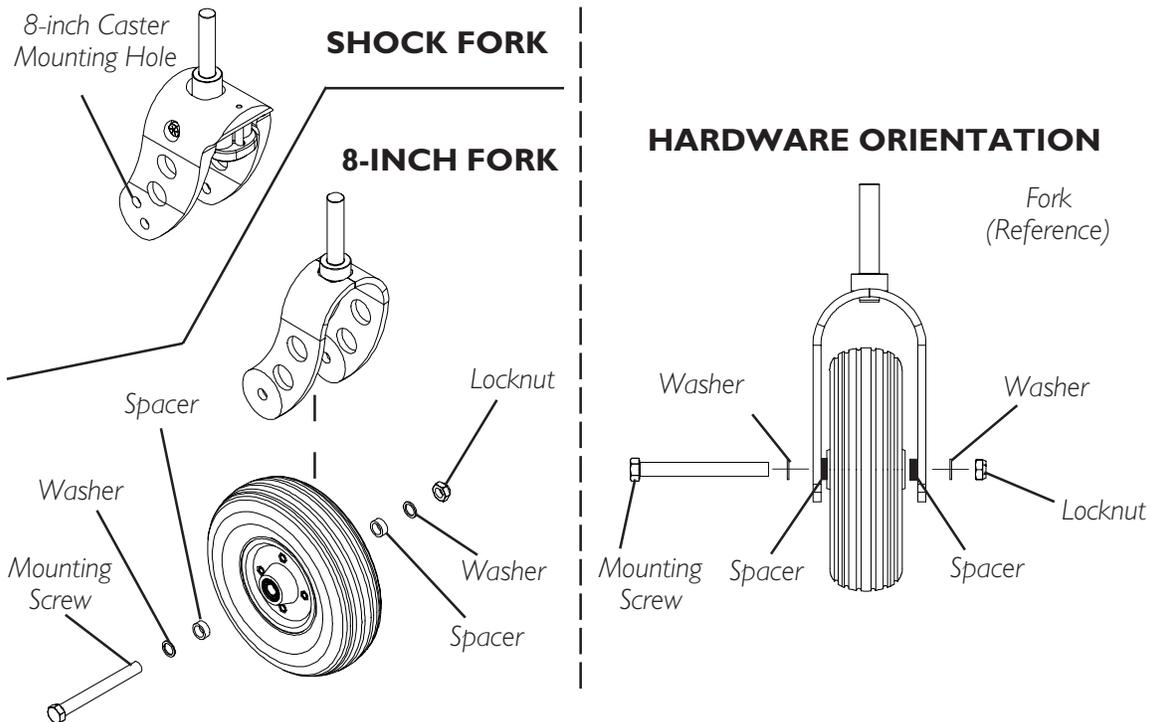
**FIGURE 7 - REMOVING/INSTALLING CASTERS**
