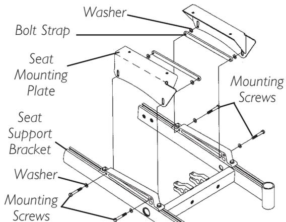
**FIGURE I - REPLACING SEAT MOUNTING PLATES**
