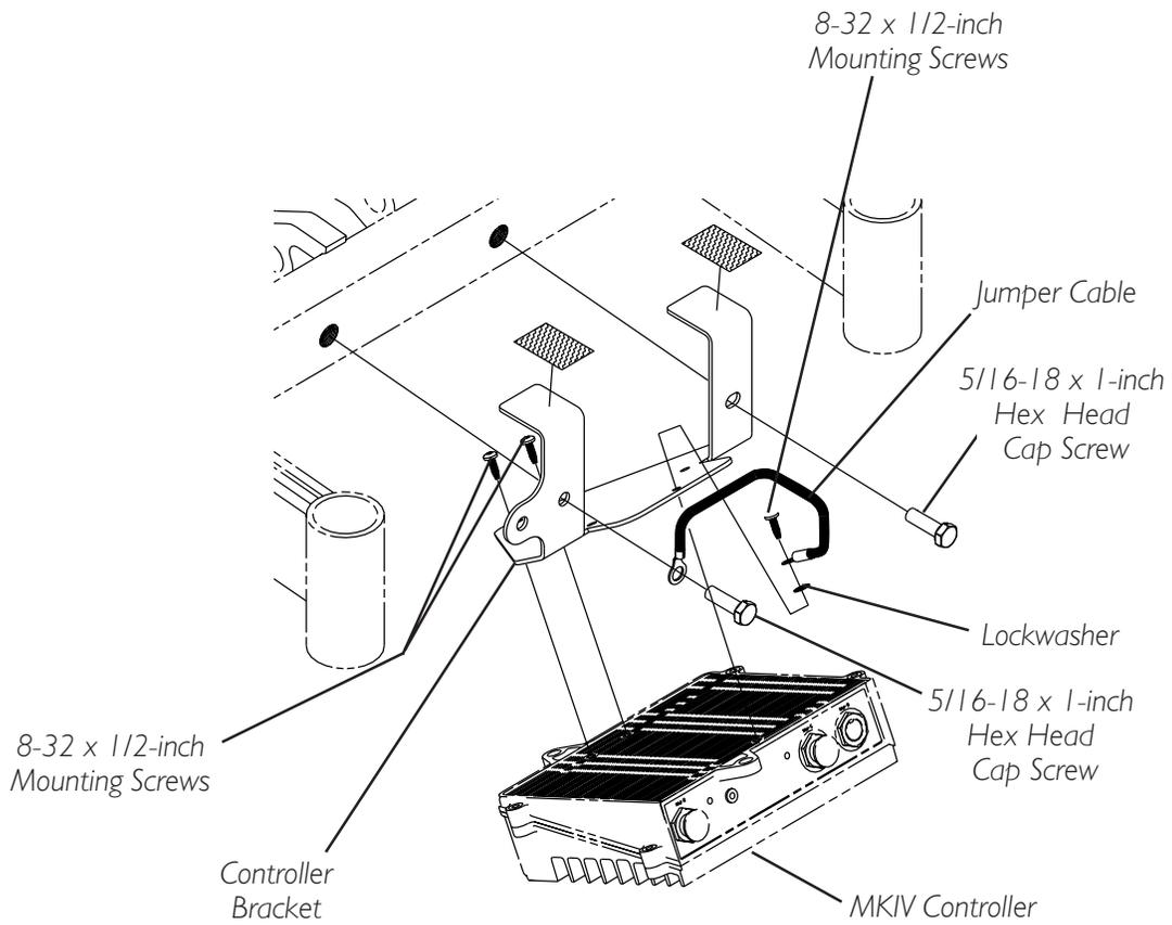
**FIGURE 2 - REMOVING/INSTALLING THE MKIV CONTROLLER
