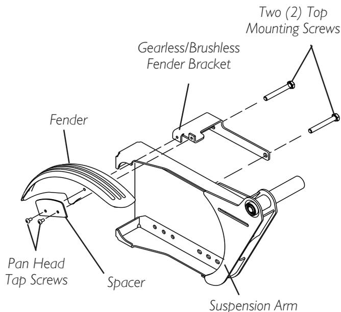
**FIGURE 13 - INSTALLING/REMOVING
