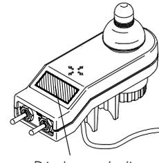
Battery Discharge Indicator (BDI) (in LCD Readout)
