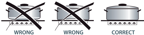
Fig. 74 Inefficient and efficient saucepan bottoms
