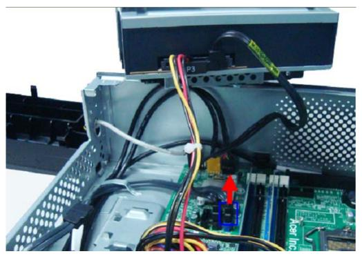
3. Disconnect the SATA (2) and power (1) cables from the rear of the hard disk drive.
