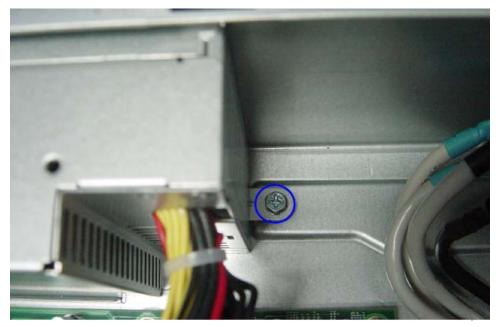
3. Remove the three screws that secure the power supply to the rear panel.
