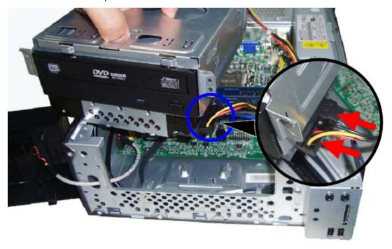
**8.** Connect one end of the SATA cable to the SATA connector on the mainboard.
