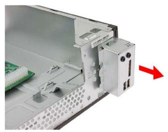
7. Remove the two screws that secure the front I/O and card reader assembly to the bracket.
