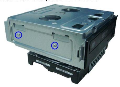
**6.** Pull the optical drive out of the drive bay.
