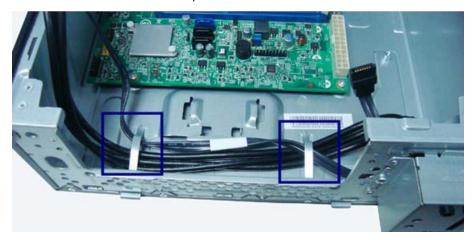
3. Disconnect the front I/O and optional card reader from their mainboard connectors.
