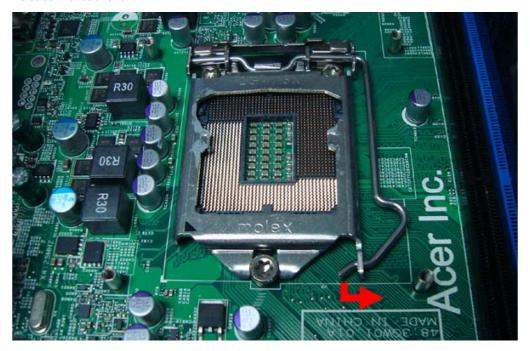
2. Lift the load lever and load plate to the fully open, upright position (1) and (2).
