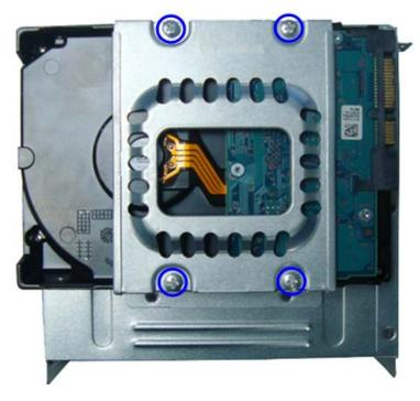
8. Slide the hard disk drive out of the bracket.
