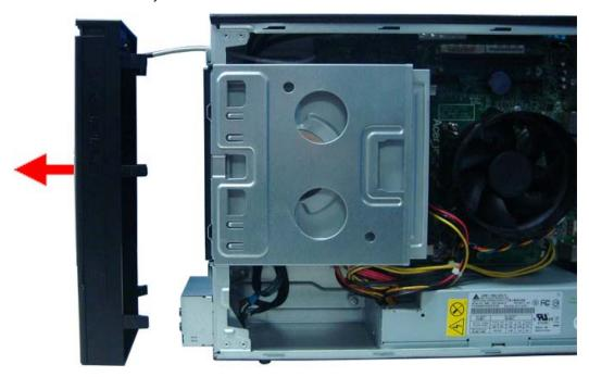
**NOTE:** The bezel can't be entirely removed until completed below step.due to the other end of power cable connecting with motherboard.
