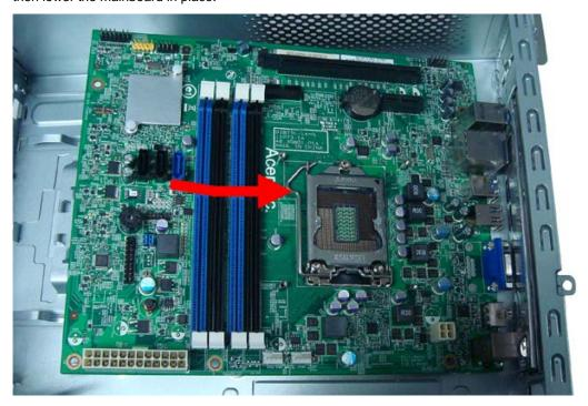
2. Make sure the screw holes on the main board are aligned with those on the chassis. Secure the mainboard with four screws.
