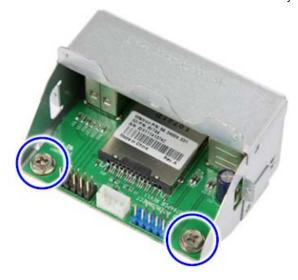
8. Remove the front I/O and card reader assembly from the bracket.
