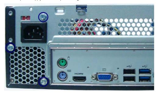
3. Secure the power supply to the chassis using the screw.
