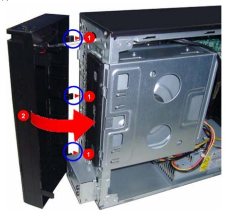
2. Make sure the front bezel retention tabs are securedly fastened to the chassis interior.
