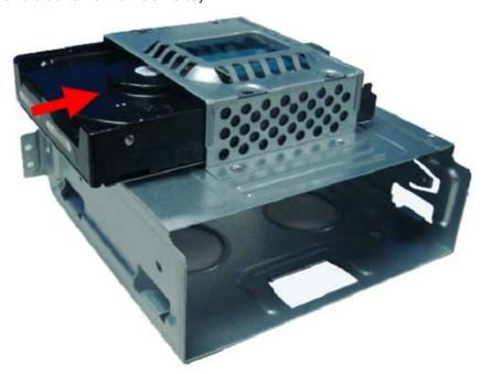
2. Secure the hard disk drive to the HDD-ODD bracket using four screws.
