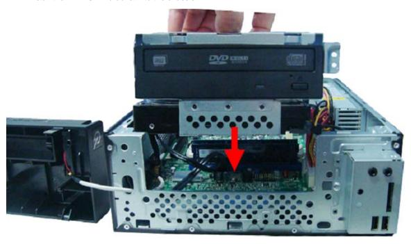
2. Secure the HDD-ODD bracket to the chassis using two screws.
