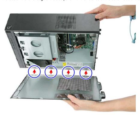
2. Align the tabs on the upper edge of the side panel with the notches on the top side of the chassis.
