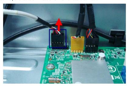
2. Pull out the power button/LED cable from the chassis.
