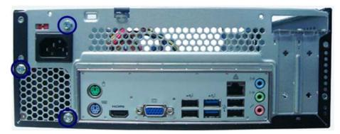
**4.** Pull the the power supply module toward the front.
