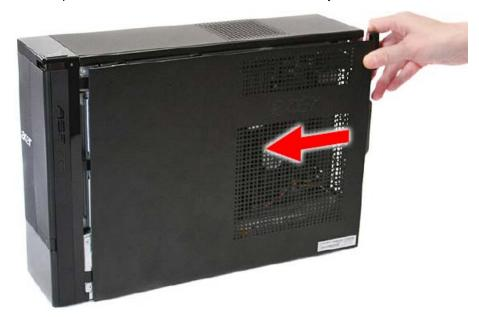
**4.** Secure the side panel to the rear edge of the chassis using two screws.
