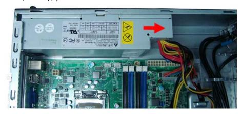
**5.** Tilt the power supply module slightly to the right and lift it out of the chassis.
