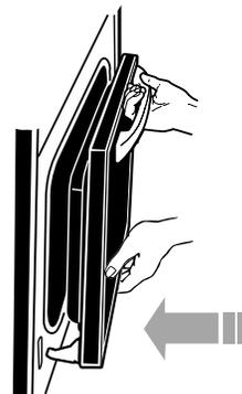
2. Open the door completely and remove the door removal pins. Save them for future use.
