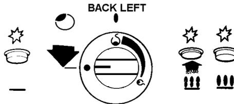
**Warning:** If the ignition button is not pressed immediately a build up of gas may cause the flame to spread.
