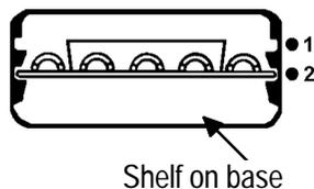
For safety the shelf will only pull out so far. If you want to remove a shelf completely, pull it forward as far as it will go, raise the front edge and lift it out. To put the shelf into a different position, keep the front edge raised, slot the shelf on to the runner, lower the front edge and slide the shelf in.
