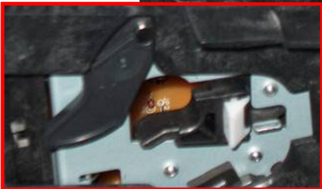
Location of cartridge alignment knob and detail
