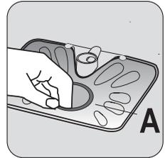
Remove filter **A** from the base of the washing compartment.
