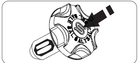
The salt cap has a refill indicator window in the centre in which a green float is clearly visible when there is salt inside the container and almost disappears when the salt has finished.
