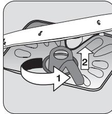
Turn the handle about 1/4 turn anticlockwise and remove filters **B** and **C**.
