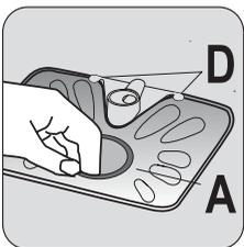
Put the flat filter **A** back in the base of the washing compartment and ensure that it fits perfectly under the two guides **D**.
