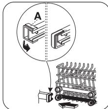
Refit the basket in the higher position and replace the stops (A) in their original position.
