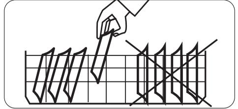
If plates are to be loaded in the upper basket: load them starting from the rear positions; tilting them slightly forwards and avoiding the front positions near the door.
