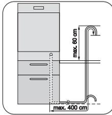
The waste connection must be at a maximum 60 cm from the bottom of the dishwasher.
