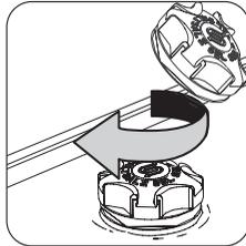
Replace the cap tightly turning it clockwise until it stops with a click.
