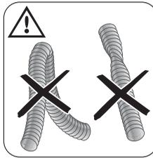
Ensure that the hoses are not kinked, crushed or entangled. The internal diameter of the couplings used for connections to the waste outlet must be no smaller than the diameter of the hose provided.
