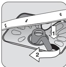
Replace the filters and lock by turning the handle clockwise to the stop.
