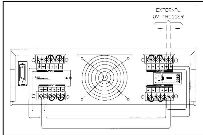
**Figure 4-7. Overvoltage Connections**
