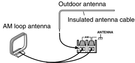
Outdoor AM antennas work best when installed horizontally outside, but good results can sometimes be obtained indoors by mounting horizontally above a window. Note that the AM loop antenna should be left connected. Outdoor antenna must be grounded in accordance with local regulations to prevent electrical shock hazards.
