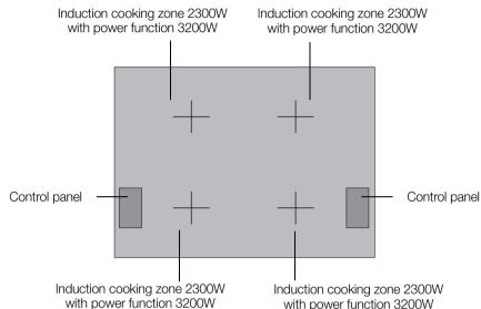
The cooking surface is divided into four cooking zones. In each cooking zone under the glass ceramic is an induction heating element, the middle of each one being marked with a cross on the glass ceramic surface. Cookware can be placed on any of the cooking zones. But
