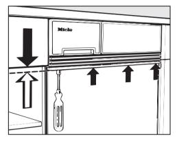
Using a socket spanner, turn clockwise or anti-clockwise until the required height is reached.
