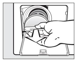
■ Unscrew the drain filter completely.
