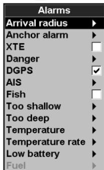
All alarms except **Loss of GPS fix** can be turned on (enabled) or off (disabled).
