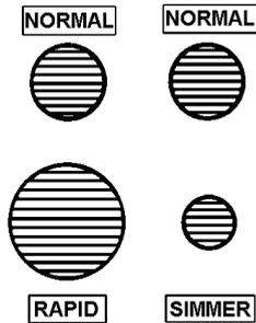
The largest pan which you should use on any burner is 230mm (9").
