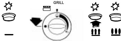
Warning: If the ignition button is not pressed immediately a build up of gas may cause the flame to spread from the grill cavity.
