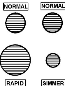
The largest pan which you should use on any burner is 230mm (9"). The base of the smallest pan should not measure less than 100mm (4").
