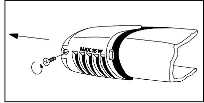
After changing the bulb replace the lamp cover, and retaining screws and reconnect the appliance to the electricity supply.
