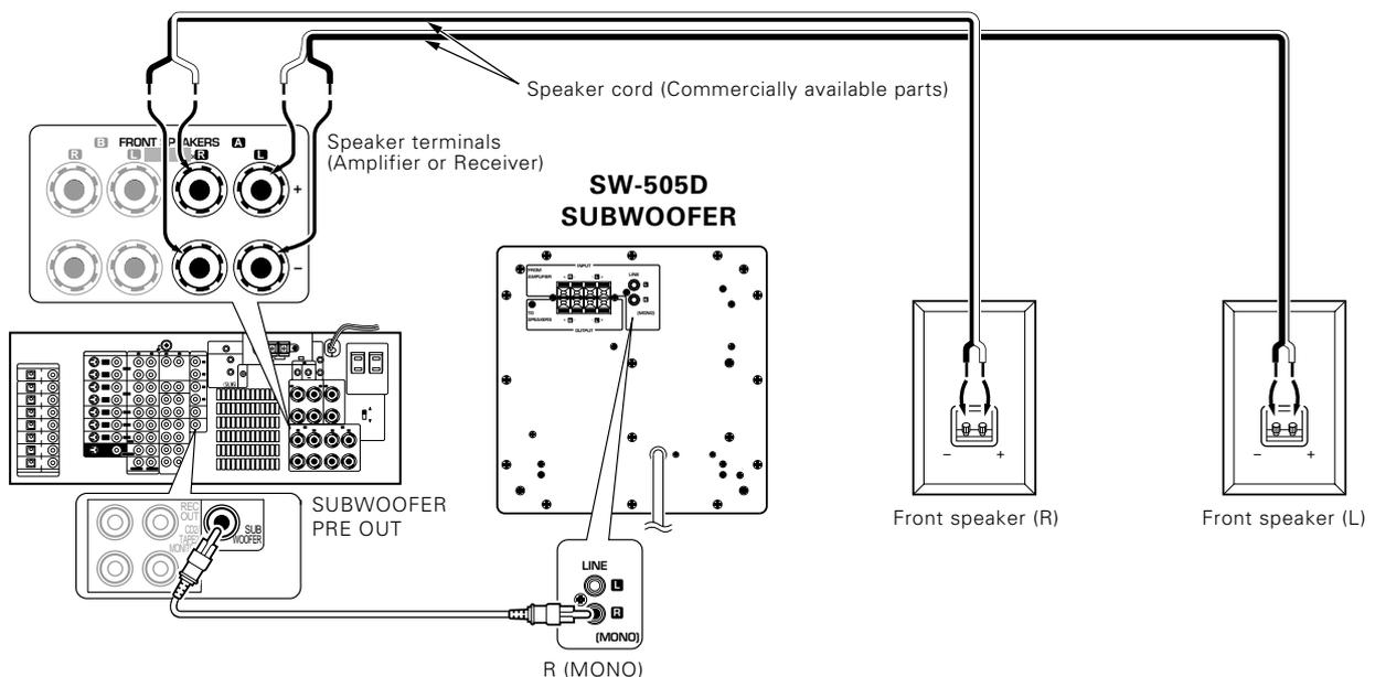
**If the amplifier is not equipped with a Subwoofer Pre-Out jack or if two subwoofers are to be used**
