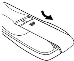
Open by pushing the position marked with the arrow.
