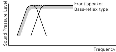
**12 dB position:** To be used when the Subwoofer is combined with acoustic air-suspension type front speakers.
