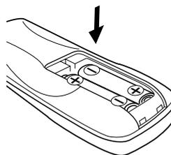
Insert two R03 ("AAA"-size) batteries according to the polarity indication.
