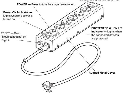
Power Shutdown Protection — Protects the connected appliances from being damaged by shutting down power when surge protection is depleted (see "Troubleshooting" on Page 2).
