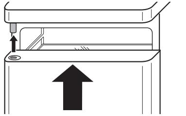
7. Place the lower door hinge bracket with the bearing pivot in the lower left of the door and fasten.
