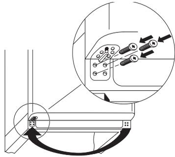
8. Unscrew the top handle bracket from the handle rod (1). Unscrew the bottom handle bracket from the door (2).
