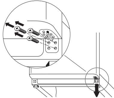
3. Remove the door fitting from the door hinge bracket (1, 2). Move the hinge bracket pivot from the right to the left hand hole (3). Place the door fitting supplied on the hinge bracket pivot (4, 5).
