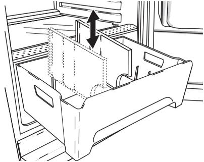
2. If the large divider is inserted in the middle of the bin the right hand side can be further divided by inserting the small divider in the middle or rear position.
