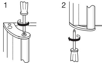
9. Unscrew the top handle bracket from the door (3) and screw onto the bottom right-hand side of the door (4).
