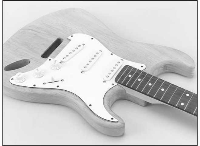
Figure 11. Pick guard alignment.
