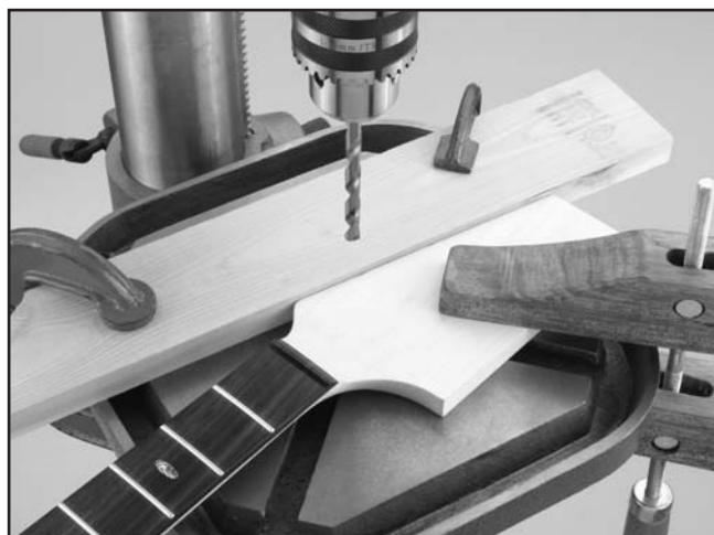
Figure 7. Drilling the pegholes.
