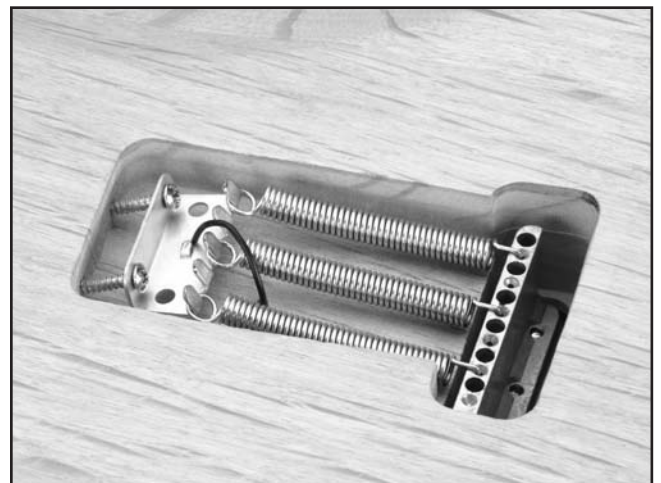
Figure 18. Correct spring placement.
