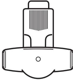
Belt clip and adapter for the handset. The adapter is clipped onto the handset and is removable without any remains or damages.
