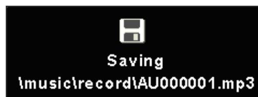
**NOTE:** The maximum length of an AV Recording file depends on hard disk free space and can not exceed 3hrs or 2GB. In Continuous mode it will make multiple files until the hard drive is full.
