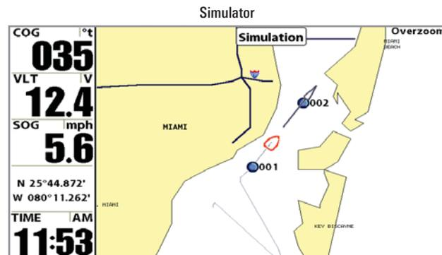
**NOTE:** At startup, while still on the splash screen (while the name of your Humminbird® model is still on the screen) you must press the MENU key and then select Simulator manually to enter Simulator mode. Manually selecting Simulator from the Start-Up Options menu allows you to pre-configure your Chartplotter for on the water operation. Any menu changes you make will be saved for later use.
