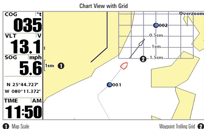
**NOTE:** Only one waypoint can have either a target or a grid at one time. If you apply a target or a grid to a new waypoint, the original waypoint will lose its target or grid.
