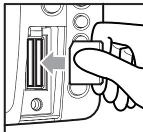
Inserting an MMC/SD
