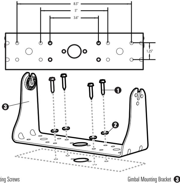
5. Set the gimbal bracket aside and drill the four mounting screw holes using a 5/32" (4.0 mm) drill bit.
