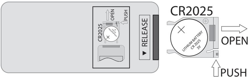
1. Push the Release Button and pull out the Battery Compartment to access the battery.
