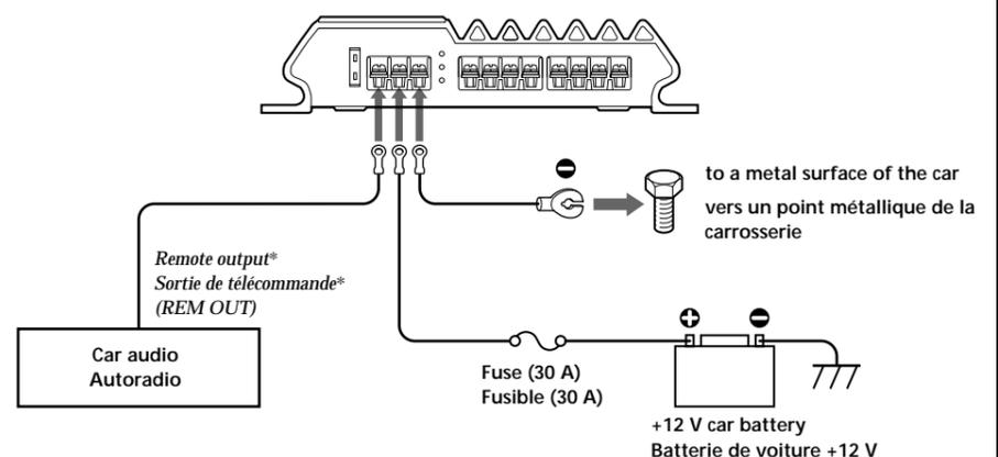
\* If you have the factory original or some other car audio without a remote output on the amplifier, connect the remote input terminal (REMOTE) to the accessory power supply.
