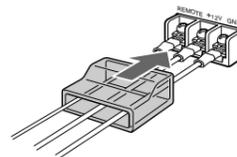
Pass the leads through the cap, connect the leads, then cover the terminals with the cap.
