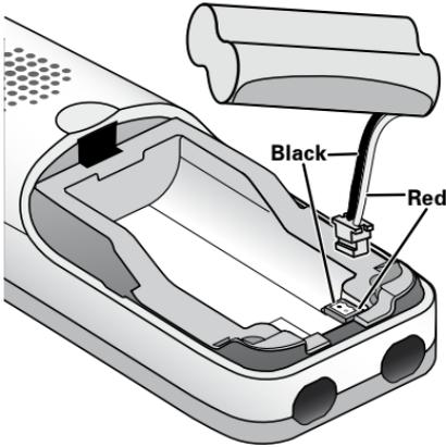
2. Line up the battery pack connector with the jack inside the handset. (The battery connector will only fit one way.)
