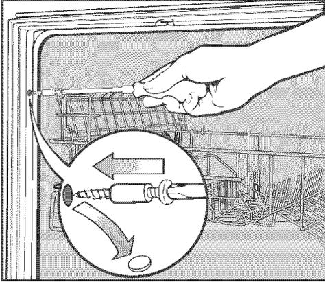
⚠ The side mounting holes should only be used for securing the dishwasher if the opening is exactly  $23 \frac{5}{8}$ " (60 cm) wide. Use of this method on larger openings can damage the machine and cause leaks. Be careful not to screw into an adjacent appliance.
