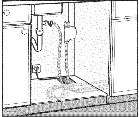
Connect the supplied drain hose to the drain pipe of the kitchen sink either:
