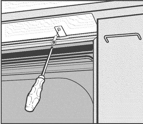
Make certain that the white rubber seal located at the top, outer edge of the dishwasher is tight against the bottom of the countertop. Do not drill any additional holes through the wash cabinet. If in doubt on how to secure the dishwasher, please call Miele's Technical Service Department.
