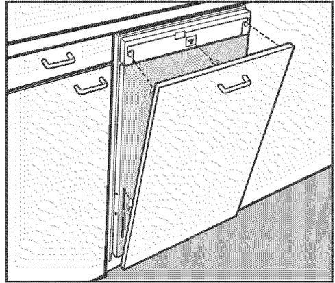
The "T" shaped hanger behind the door handle should fit easily into its respective hole.
