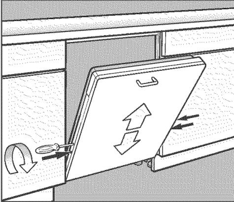
Adjust one side of the door panel at a time using a T20 Torx screwdriver.
