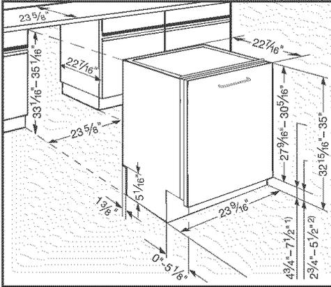
Machine heights of 35" - 37" (889-940 mm) cannot be obtained using the supplied legs. For this height range, or for heights greater than 35" (889 mm), extended legs (part# 02 702 601) are necessary. Contact the Miele Technical Service Department for the appropriate legs.
