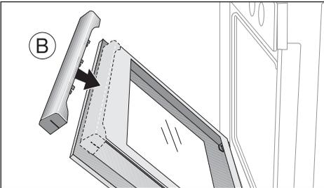
pushed **between** the outer door panel and the guide corner (D).
