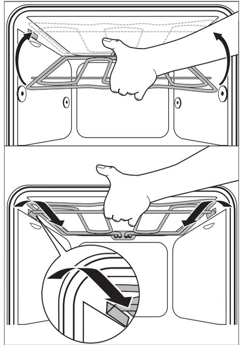
1. Move the heating element back up towards the oven ceiling.
