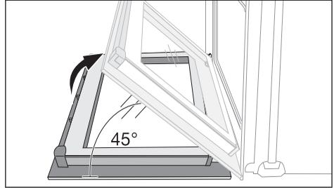
4. Take hold of the oven door with a hand on each side and pull it away from the oven at an upwards angle (**Take care: It is heavy**).
