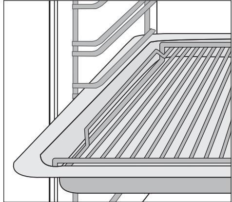
The grill tray rests on the roasting pan. Push the roasting pan between the guide bars of the selected oven level.
