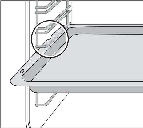
Push the roasting pan between the guide bars of the selected oven level.
