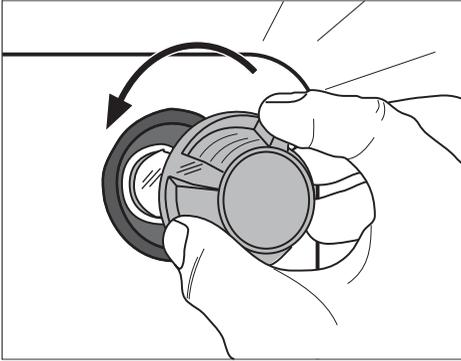
1. Remove the glass cover by turning it anti-clockwise and then clean it.
