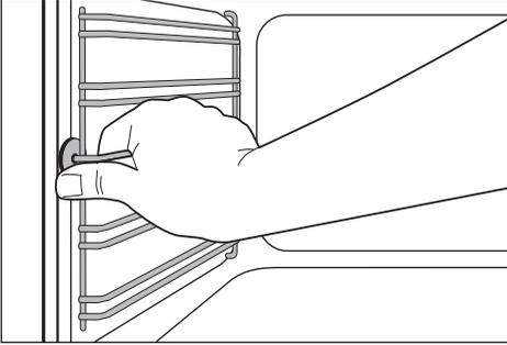
First pull the front of the rail away from the oven wall (1) and then unhitch at the back (2).
