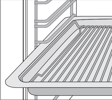
The grill tray rests in the roasting pan. Push the roasting pan between the guide bars of the selected oven level.
