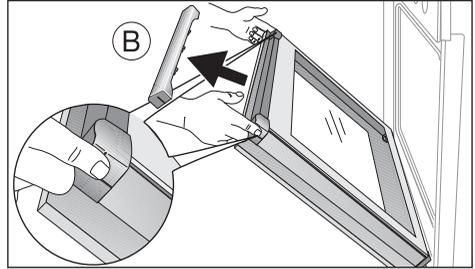
5. Take hold of the door glass on its upper edge and take it out of the guide by pulling it upwards.
