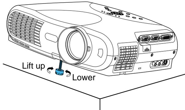
**Turn the foot adjuster to make fine adjustment to the height.**
