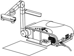
**Set the white paper on a flat surface and set the camera so that the paper is projected onto the screen.**
