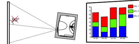
Select "H-keystone" from the menu with the selection buttons (▲/▼), and adjust the distortion of the upper and lower sides of the picture with the selection buttons (◀/▶).
