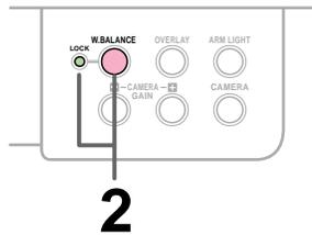
This projector's camera is always being adjusted automatically for projected color balance; however, the balance can shift away from optimum due to the color scheme of the document. Should this occur, the white balance can be set to a fixed condition by using the following procedure.
