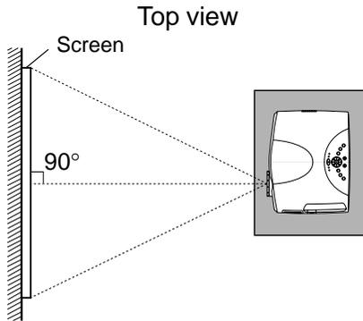
Point the lens straight at the center of the screen as above.
