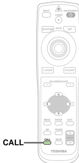
Information on the input signal source, etc., can be displayed.
