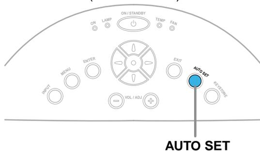
You can adjust the optimum horizontal position, vertical position, sampling phase and sampling frequency for projecting analog RGB signals at the touch of a button.
