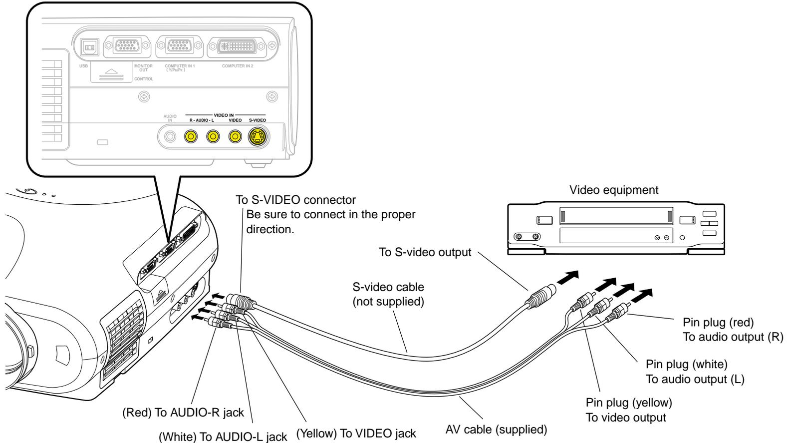
**Note** The S-VIDEO connector and VIDEO jack can be used independently, but the audio input jacks are used as both the S-VIDEO and VIDEO input.
