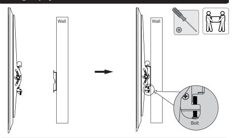
Tighten the two bolts by using an appropriate phillips screwdriver to secure bracket.
