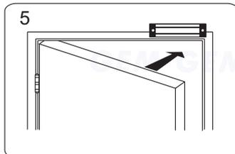
5 Close the door. Measure the correct position by bringing the armature plate close to the contact surface of the electromagnetic lock.
