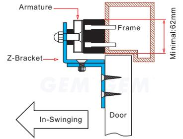
■ Application for the Electromagnet: GL-1200 series
