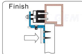
Finish Once the position is correct, use the screws to permanently mount the Z bracket on the door frame. This should be the last step.
