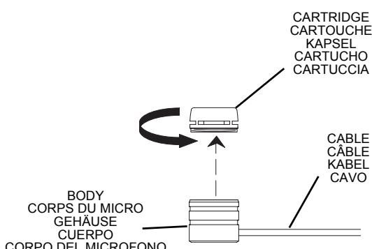
REMOVING A MICROPHONE CARTRIDGE
