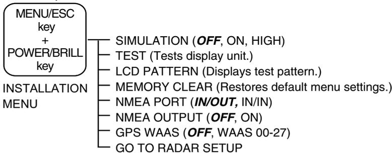
Choose GO TO RADAR SETUP from the INSTALLATION menu, and then go to page 4 of the SYSTEM menu.
