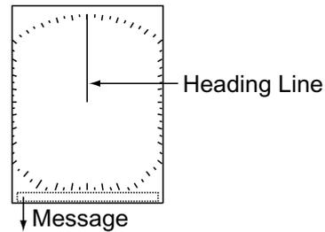
HEADING LINE ADJUSTMENT BY '◀' AND '▶' KEYS. THEN PUSH MODE KEY TO SET.
