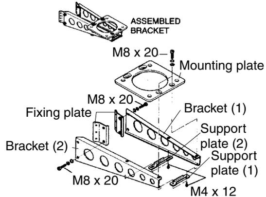
**(A) Assembling the mounting bracket**
