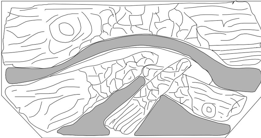
Remove the ember material from the plastic bag. Cover the shaded areas in the diagram shown beside. Totally fill these areas with glowing ember material.
