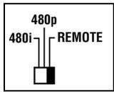
If you want to select the scan mode between the interlace and progressive modes depending on the source condition or when connecting more than one television, you can select the mode from the remote control unit. To do this, set the scan mode selector on the rear panel to "REMOTE" (See page 7).
