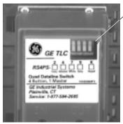
To access the Master Button DIP switches, remove the gray portion in the upper right corner of the label on the back of the dataline switch.
