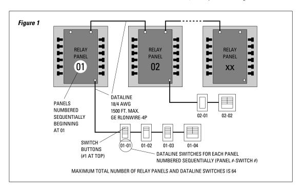
Any switch button may be softwired to control a single relay or a group of relays within any single panel (see next page for softwiring a dataline switch). For example, assume that you want the top two buttons of a 4-button switch to control open office areas associated with relays in Panel 01, while the
