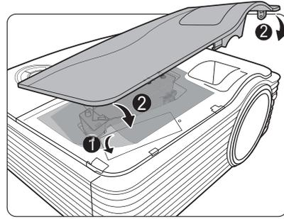
14. Tighten the screws that secure the lamp cover.
