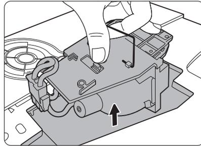
8. Insert the new lamp into the lamp compartment and make sure it fits in the projector.
