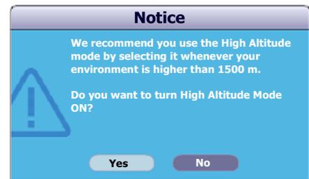
Operation under "**High Altitude Mode**" may cause a higher decibel operating noise level because of increased fan speed necessary to improve overall system cooling and performance.
