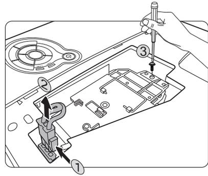
7. Lift the handle so that it stands up. Use the handle to slowly pull the lamp out of the projector.
