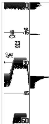
The **Wide RTS™ Window** indicates the sonar intensity through the use of a bar graph. The length of the plotted return provides an indication of whether the return is weak or strong. The depth of the sonar return is indicated by the vertical placement of the return on the display depth scale. The Wide RTS™ Window does not make use of grayscale.
