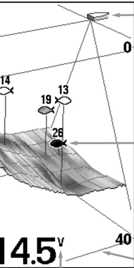
**Boat/Direction Arrow** - A simple, solid 3D boat is drawn when the Upper Depth Range is 0. A solid 3D arrow is drawn when the Upper Depth Range is not 0.
