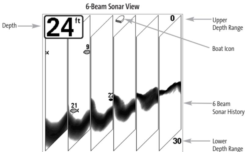
The digital readouts in the 6-Beam Sonar View cannot be customized, making information such as water temperature and voltage unavailable in this view.
