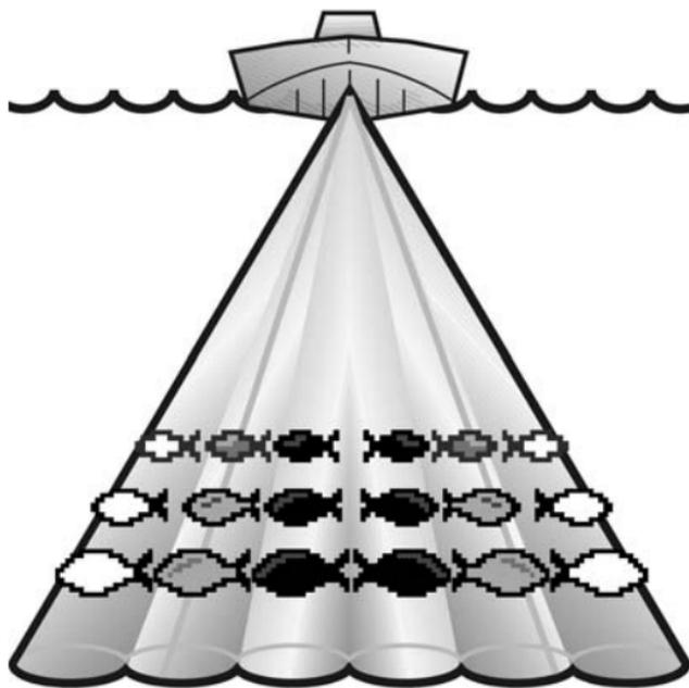
When Fish ID+™ is turned off, the Fishing System shows only the raw sonar returns on the display.
