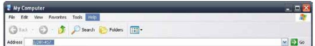
**Step 2** Input \\ followed by the Storage Server name or the IP address of the router in the URL input text box (\\DIR-457 or \\192.168.0.1). (you can enter default Storage Server name or user-configured name ).
