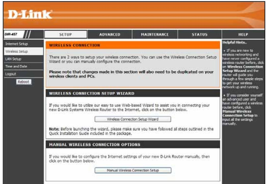
Click the **Wireless Connection Setup Wizard** button to view the **Wireless Security Setup Wizard** menu. The Welcome menu lists the steps used for setup. Click on the **Next** button to continue.
