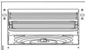
1. When cooking on two levels use both the shelves supplied, with the square tray on the lower level and the square rack on the upper level.
